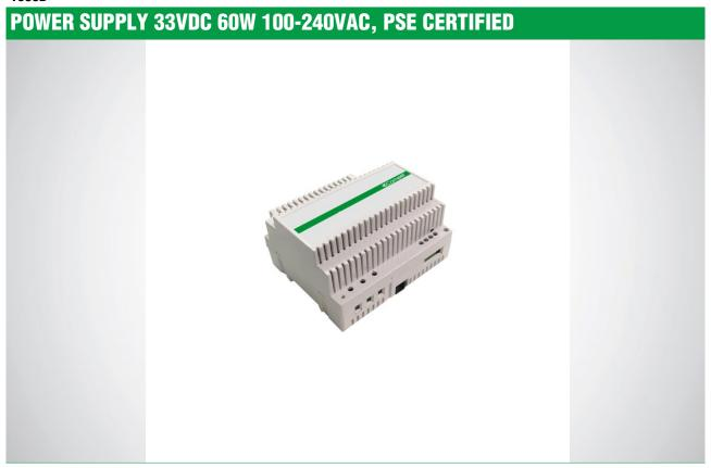
Power supply unit with 110-230 VAC primary and 33 VDC / 1.8A continuous output for 316 range entrance panels. Equipped with internal protection against current overload and short circuits. Dimensions: 106x89x62 mm (6 DIN modules). PSE certified.
