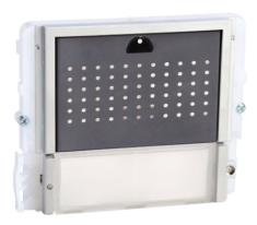
Module designed for audio speaker unit, with stainless steel finish faceplate. Nameplates with LED lighting (options: blue, white or off). To be fitted with an audio speaker unit depending on the cabling system used. Dimensions 112x89.5x32 mm.
