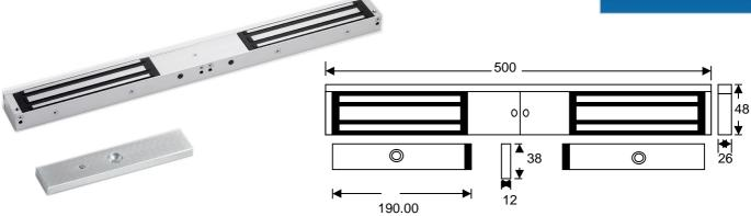
The EM04 series lock is a surface mount "face to face" electro-magnetic lock offering up to 275kg of holding force per leaf \* these locks can be used on either out-swing or inward opening doors.
