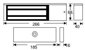
The EM10 series lock is a surface mount single "face to face" electro-magnetic lock offering up to 1200lb of holding force these locks can be used on either out-swing or inward opening doors.
