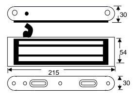
The EM750R magnetic lock is totally sealed in an epoxy sealed stainless steel case for water-resistant and vandal-resistant purpose. Offers up to 800lb holding force. It can be applied with access control.
