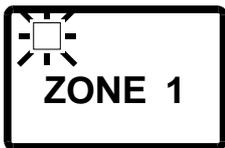
Green indicator flashing. A detector has activated the lighting for a zone.
