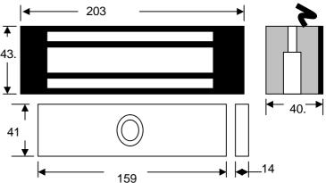
The G600S & G600SM magnetic lock is totally sealed in an epoxy sealed stainless steel case. Up to 800lb holding force. It can be applied with access control.
