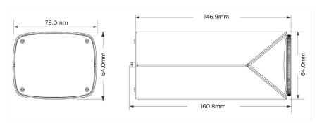
The VA Analogue 1/2.8" 2MP IP Box Camera serves as a visible deterrent whilst offering enhanced image quality through a wide dynamic range feature.
