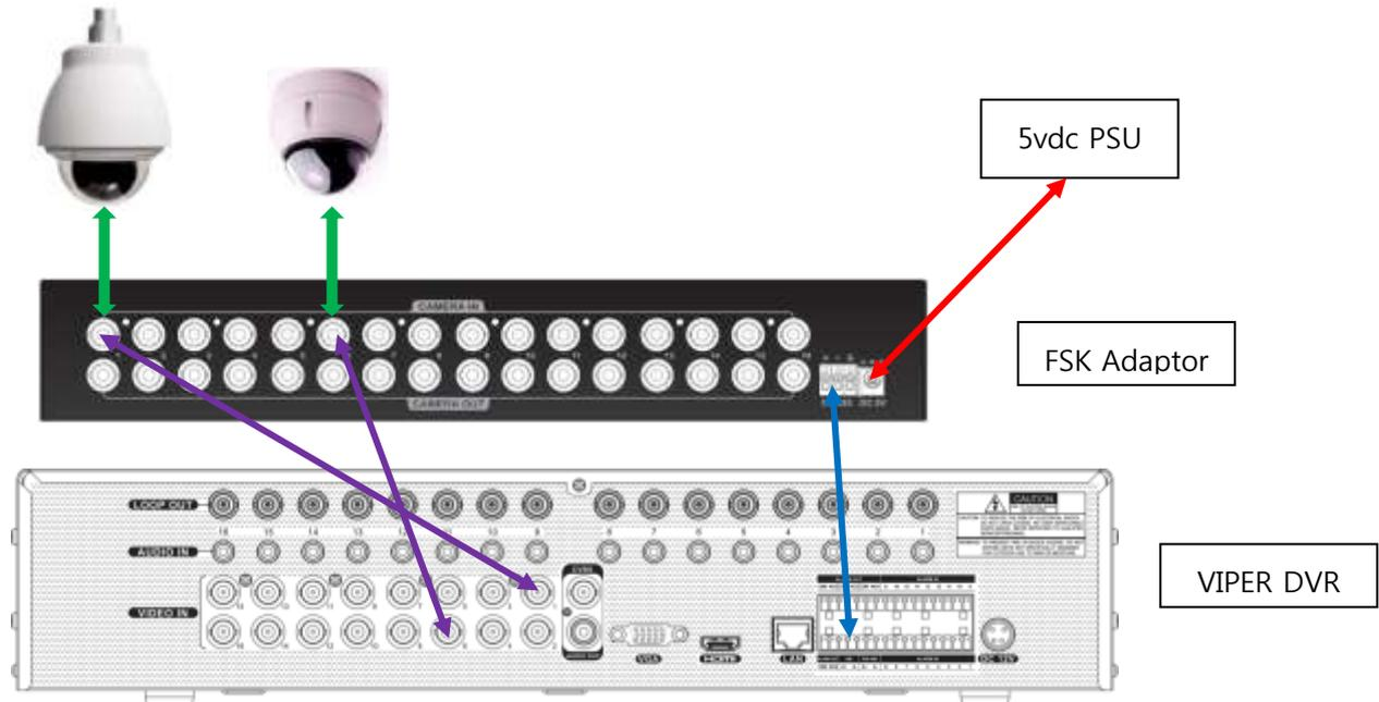
1. Connect the **coax** cable from the PTZ dome to the CAMERA IN on the FSK Adaptor.
