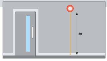
Unless MICC cable is used, all cabling should be mechanically protected from floor level up to a height of 2m.
