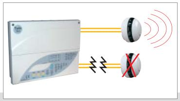
Sounder device cabling should be arranged so that in the event of a fault at least one sounder will remain operational during a fire condition.
