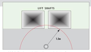
Vertical shafts like lifts and stairways should have a device mounted within 1.5m of any opening.
