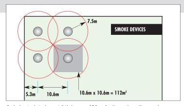
Smoke detection devices have an individual coverage of 7.5m radius. However these radii must overlap to ensure there are no 'blind spots'. Therefore the individual coverage can be represented by a square measuring 10.6 x 10.6 m giving an actual area coverage of  $112 \text{m}^2$  per device.
