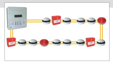
Short circuit isolators limit the effect of one fault to 2000m². '2 simultaneous faults on a circuit should not disable protection within an area greater than 10,000m². With the Sita 200 Plus the isolator is built in to every device for maximum protection.
