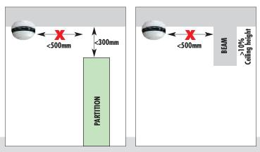
A device should not be mounted within 500mm of any obstruction.
