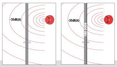
Decibel loss occurs through doors: approximately -20dB(A) through a normal door, and approximately -30dB(A) through a fire door.
