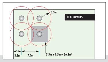
Heat detection devices have an individual coverage of 5.3m radius. However these radii must overlap to ensure there are no 'blind spots'. Therefore the individual coverage can be represented by a square measuring  $7.5 \times 7.5m$  giving an actual area coverage of  $56.3m^2$  per device.
