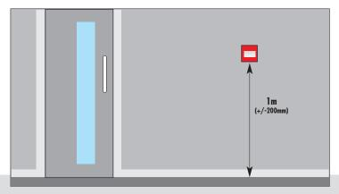
Manual call points should be positioned between 800mm to 1200mm from floor level.. Any non-mechanically protected cable medium should have additional protection up to a height of 2m from floor level.
