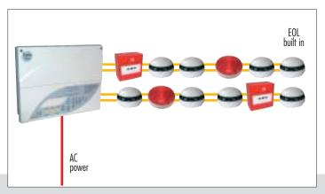
Fire resistant cabling is now required within the whole fire alarm system including the mains supply cables. The use of non-fire resisting cables whether mechanically protected by fire-resisting construction or not, will no longer comply with BSS839. With the Twinflex system, separate sounder units are not required as each zone incorporates a sounder unit.
