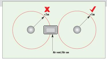
Don't site detectors less than 1m from air Inlets or air conditioning units.
