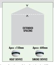
For ceilings that feature a apex: as long as the height of the apex from the rest of the ceiling is less than 150mm for Heat detectors or less than 600mm for Smoke detectors then these can be treated the same as flat ceilings. For higher apexes, a device should be installed at the highest point. The distance to adjacent devices can be increased by 1% per degree of angle of the roof up to a maximum of 25%.
