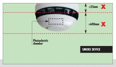
The sensing element of a Smoke detection device (photoelectric smoke chamber) should not be less than 25mm below ceiling, and not greater than 600mm below ceiling.
