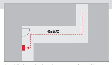
A person should not have to travel more than 45m along an escape route to reach a Manual Call Point. (25m if disabled person to operate, or rapid fire development is likely). Manual Call Points should be sited at all stair wells and exits from the building.
