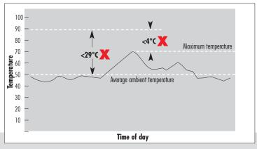
The minimum static response of heat devices should not be less than 29°C above the average ambient temperature, or less than 4°C above the highest temperature the device can be expected to experience.
