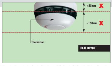
The sensing element of a Heat detection device (thermistor) should not be less than 25mm below ceiling, and not greater than 150mm below ceiling.
