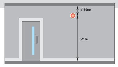
Visual alarms such as strobes should always be mounted above 2.1m from floor level but never closer than 150mm to the ceiling.
