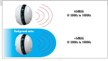
The minimum sound level of a sounder device should be 65dB(A) or 5dB(A) above a background noise which is louder than 60dB(A) (if lasting more than 30 seconds) and at a frequency of between 500Hz and 1000Hz. The maximum sound level should not be greater than 120dB(A) at any normally accessible point. May be reduced to 60dB(A) in stairways, enclosures up to 60m² and specific points of limited extent.
