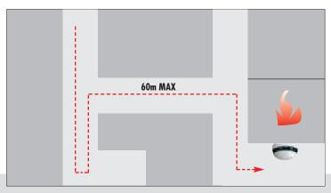
A person searching a Zone for a fire should not have to travel more than 60m to identify the source of a fire.
