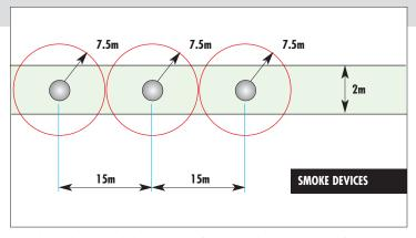
In corridors less than 2m wide the horizontal spacing of detectors may be increased, the areas of coverage need not overlap as in the case of a room.
