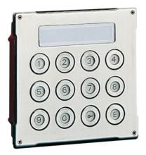
Made using double 2.5 mm 316 stainless steel plate. Complete with backlit keypad. Features 300 different 8-digit codes that can be programmed from the keypad to control two relays (10A), as well as a confirm request buzzer and relay activation LED. Relay closure time can be set from the keypad. Dimensions:  $106 \times 106 \times 56$  mm.
