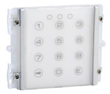
Digital electronic key module with LED keypad backlighting. Blue, white and off lighting options. When a number with between 1 and 8 digits is entered on the keypad, two relays (10A) are activated, allowing the operation of electric door locks or other devices. Dimensions 112x89.5x40 mm.
