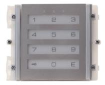
Digital electronic key module with LED keypad backlighting. Blue, white and off lighting options; stainless steel finish. When a number with between 1 and 8 digits is entered on the keypad, two relays (10A) are activated, allowing the operation of electric door locks or other devices. Dimensions 112x89.5x40 mm.
