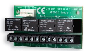
The 8600 relay expansion card is designed to fit a range of Eaton security equipment converting transistorised inputs to clean contact relay inputs. This card contains eight relays, each with its own dedicated input.
