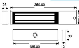
The EM01 series lock is a surface mount "face to face" electro-magnetic lock offering up to 275kg of holding force\* these locks can be used on either out-swing or inward opening doors.
