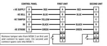
The following diagram illustrates how to wire multiple units together:
