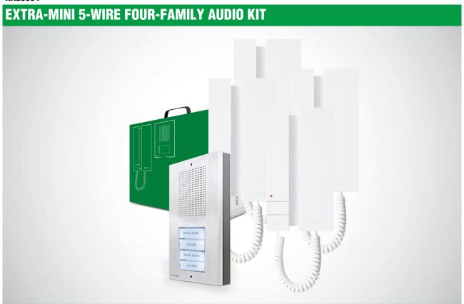
The kit includes: four Mini series door-entry phones art. 2702W, a transformer art. 1200, an Extra series external unit designed for 2/4 call buttons art. ET5100, 4 single buttons for Extra entrance panel art. ET9211. The kit can be expanded with another door-entry phone for each user. The external unit can be surface-mounted or flush-mounted using the corresponding accessories supplied with the kit.
